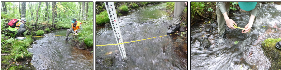
Figure 57. Documenting a typical channel cross-section at the head of riffle at Pre-emption Creek: measuring active channel width (left), active channel depth (center), and feature material (right)
