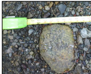
Figure 52: Particle Median Axis Diagram (left); measuring the median axis of a cobble at Halls Brook (right)
