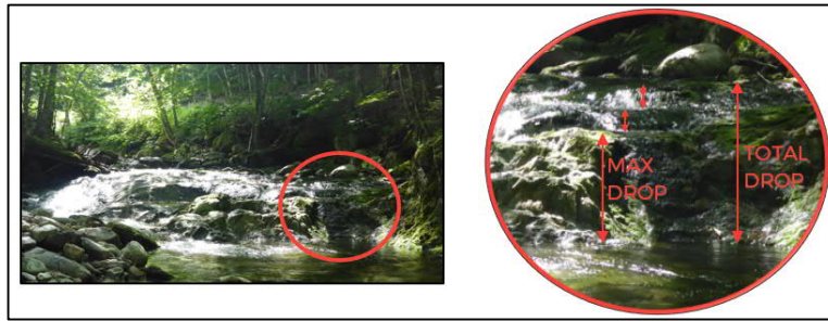
Figure 60. Feature with varying maximum drop and total drop on White River bedrock cascade
