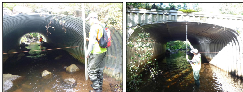
Figure 80: Field team uses the range finder function on the digital Clinometer to measure distance from cross section to upstream face of culvert on Pre-emption Creek (left) and a field member measures the distance from the line level to the crown of pipe on W. Branch Knife River (right)
